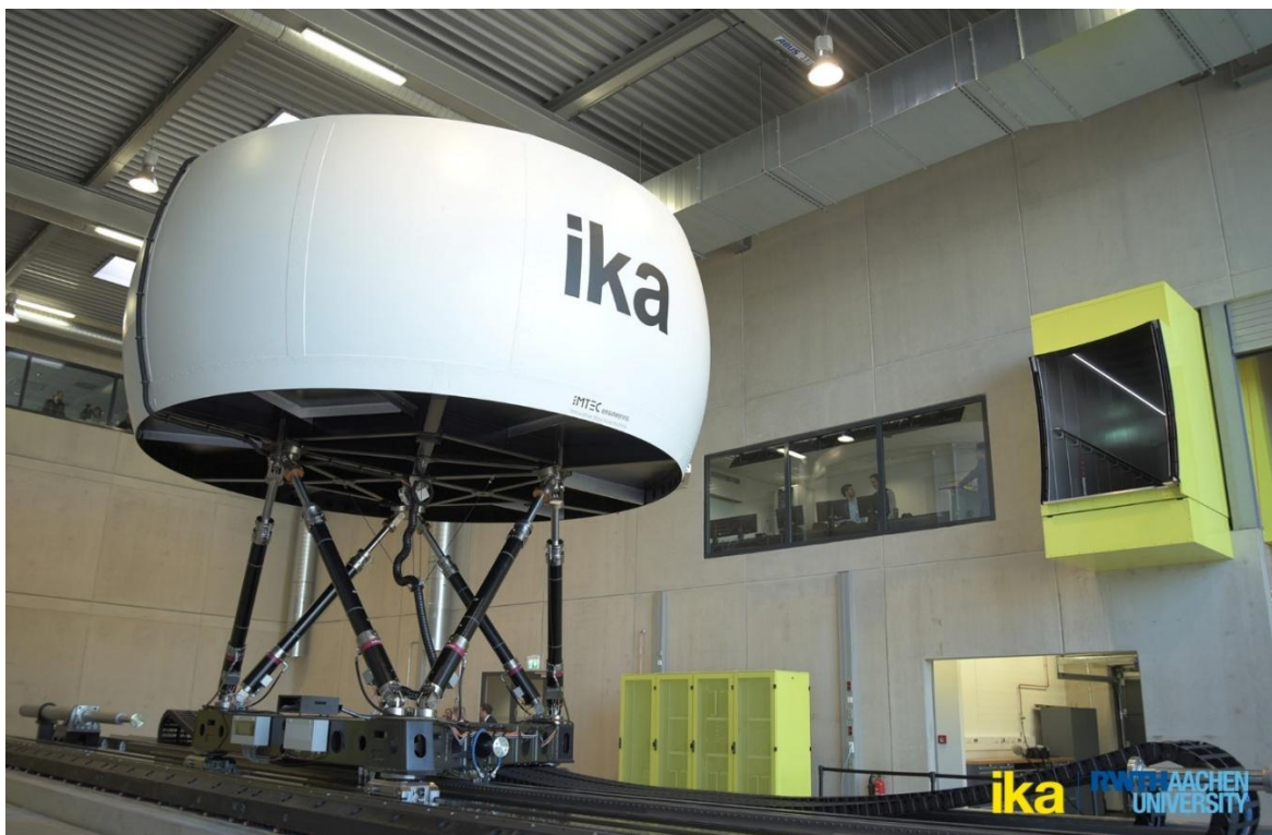
Figure 23: ika's highly dynamic driving simulator [69]
